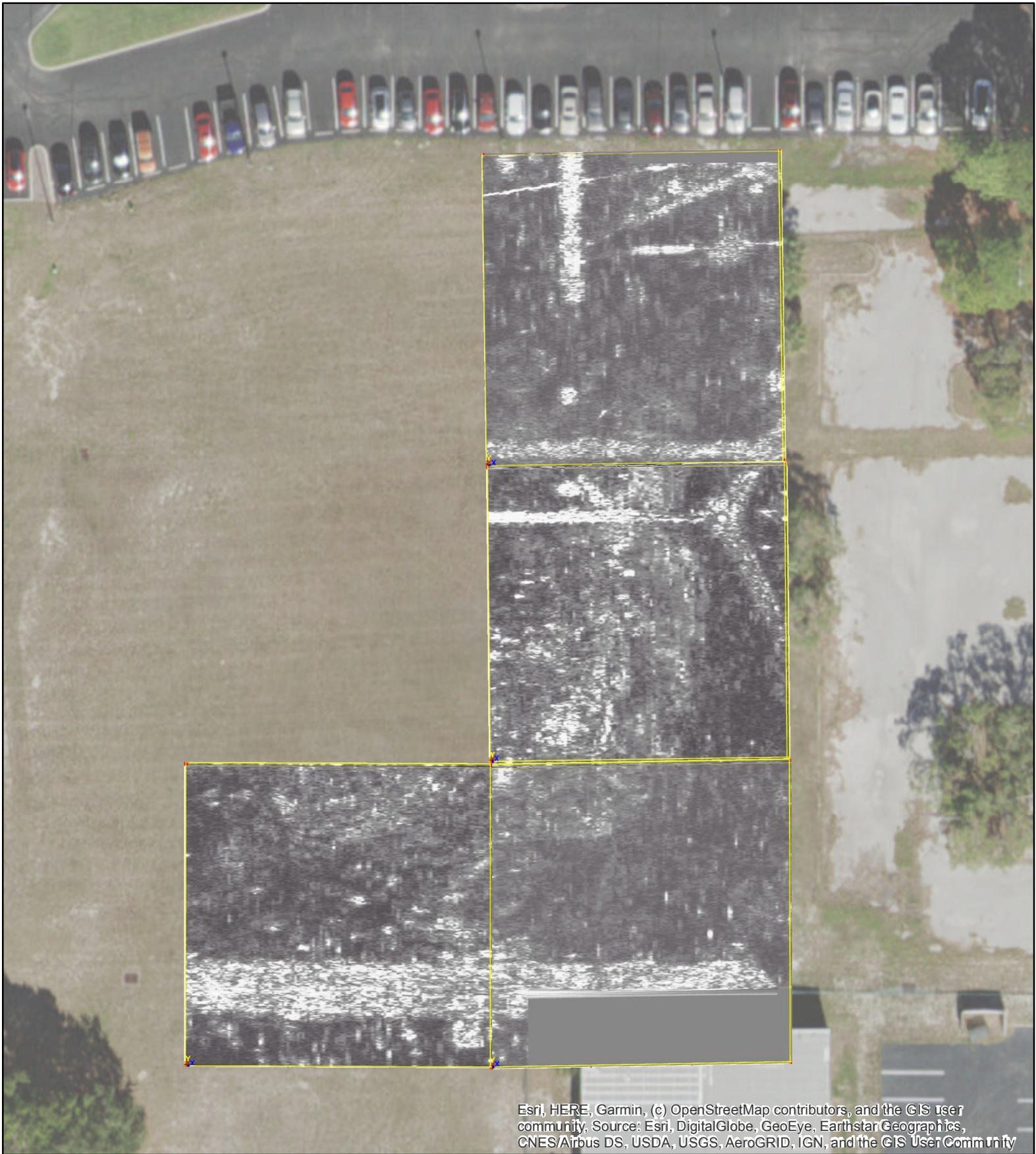
Figure 2: GPR results for grids 1-4 at 110 cm below the surface.
